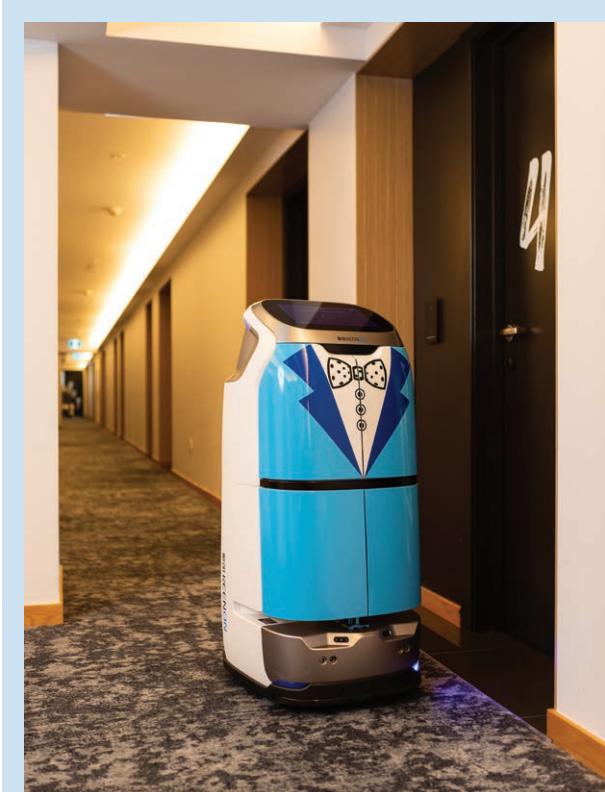
H.A.R.I. can fit a wide variety of items from food and drinks to towels and amenities. It currently can run 4 errands in succession. H.A.R.I. is interfaced with both the elevator and phone systems which allows him to take the elevator autonomously then alert the guest upon arrival to their room.
