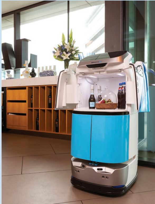
H.A.R.I. can fit a wide variety of items from food and drinks to towels and amenities. It currently can run 4 errands in succession. H.A.R.I. is interfaced with both the elevator and phone systems which allows him to take the elevator autonomously then alert the guest upon arrival to their room.
